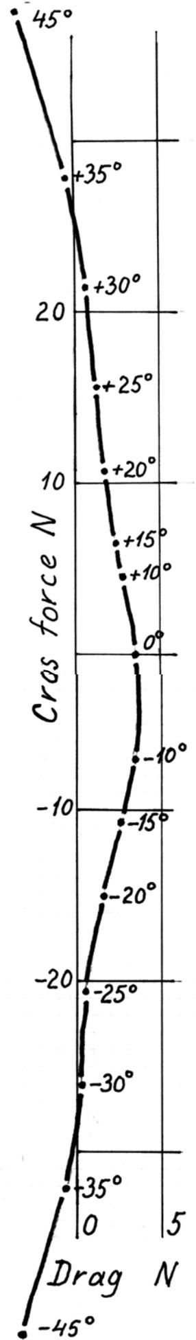
Fig. 3. Forces on a 1:5 scale model of the Leitra "Sport" at 32 m/sec.
