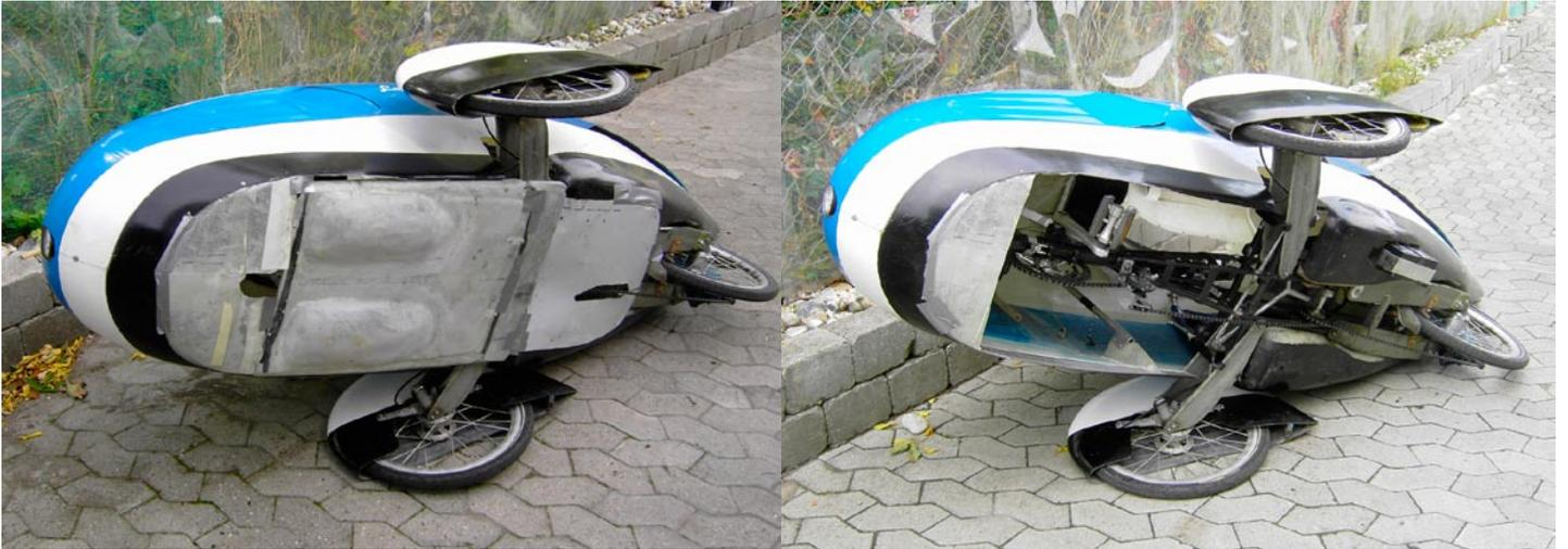
Fig. 9. Leitra "Sport" fairing with and without closed bottom.
