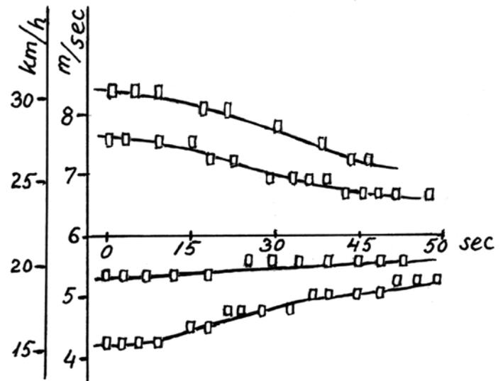
Fig. 6. Recording of speed as a function of time, measured by coasting down a 1.3 % slope on rough asphalt with Schwalbe Maraton + tyres at 5 bar. No wind.
