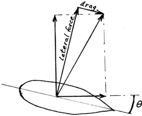
The diagram with direct measurements can be transformed into an other diagram, which shows the forces as drag and lateral force at different angles of incidence, see right side of Fig. 2 and Fig. 3.
